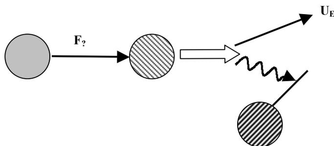
1.2.4. Useful and harmful effects exist in a system in which the elements  $S_1$  and  $S_2$  must be in contact. Counteract the harmful effect of  $F_1$  by having  $F_2$  neutralize the harmful effect or gain an additional useful effect. *Examples:*
