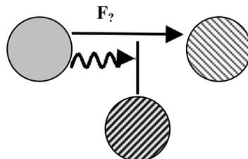
1.2.2. Similar to 1.2.1., but new substances cannot be added. Remove the harmful effect by modifying  $S_1$  or  $S_2$ . This solution includes adding “nothing”—voids, hollows, vacuum, air, bubbles, foam, etc., or adding a field that acts like an additional substance. *Examples:*
