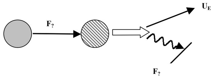
1.2.5. A harmful effect may exist because of magnetic properties of an element in a system. The effect can be removed by heating the magnetic substance above its Curie point, or by introducing an opposite magnetic field.
