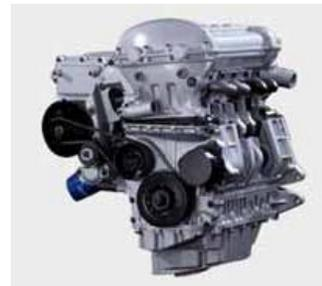
the compression ratio. The SVC engine can be run at the optimum compression ratio of 14:1 at low load and lowered to 8:1 at high load with supercharging (225hp, 224 lb.-ft./1.6L). This concept reduces fuel consumption by up to 30% when compared to a larger conventional NA engine of similar power output. (<http://www.saabnet.com>)
