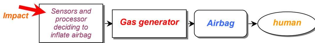
Superfluous action of airbag speaks about functional excess of gas generator and the system in the whole. Therefore a new generation of expensive cars is supplied multi-step gas generators which will fill airbags with portion of gas proportional to force of impact. This adjusting methodology improves situation, but does not solve a problem. The danger of false "undermining" of charges still remains.
