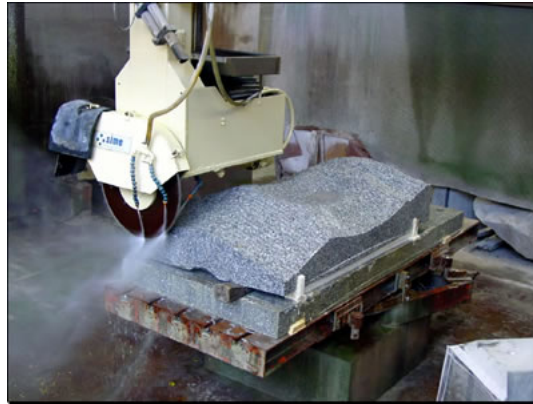
Execution of the apse capital in granite stone © Junta Constructora del Temple de la Sagrada Família
