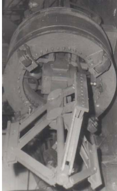
Fig. 5. Module with rubber plugs for Testing Reinforced concrete pipes diameter 1200 mm.
