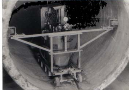
Fig. 9.a General Look of the Spraying Device Inside a Pipe
