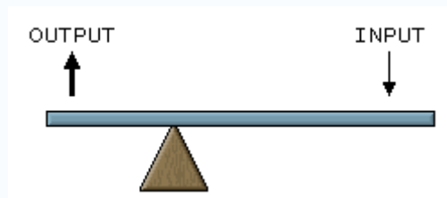
Fig.5. General Scheme of a First Class lever
