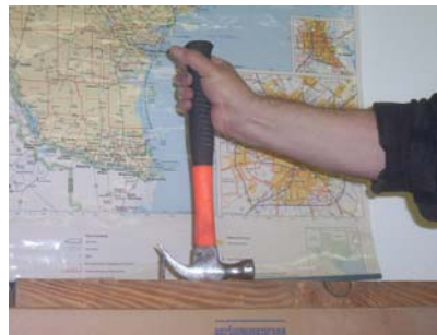
Fig.11. Nail extracting hammer is a lever
