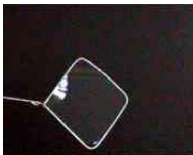
Fig.1. Plane wire frame after immersing in soap solution and taking it out
