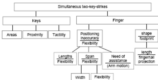
Modification of the keys-section of the OAF diagram for the keyboard too large unwanted effect.
