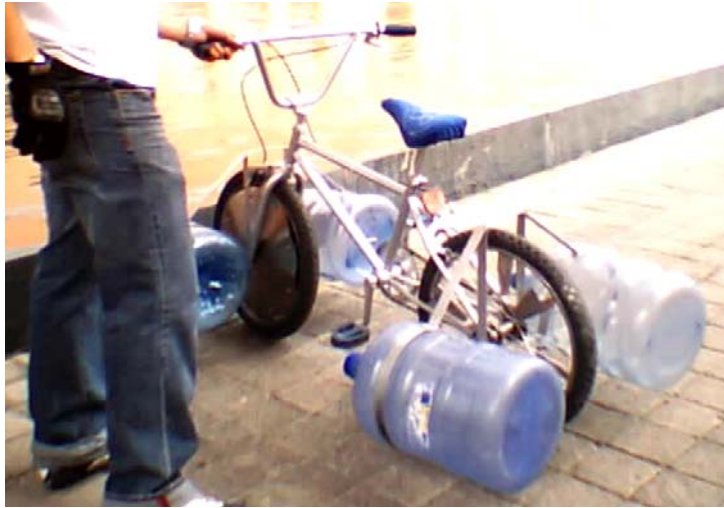
Figure 4: The winning model on land. Notice the extra fins (partially folded metal sheets) attached to the spikes of the real wheel. The front wheel is covered to facilitate turning.
