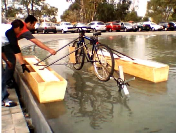
Figure 8: The other proposal with a big propeller, the size of which was still not sufficient to push the whole system and hence broke after a few minutes of ride.
