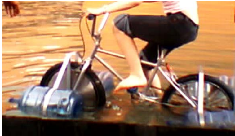
Figure 6: Side view of the winning model in water. Once again notice the extra fins (partially folded metal sheets) attached to the spikes of the real wheel.
