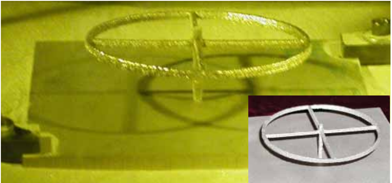
Figure 1: Patent-Pending LENS Geometry Breakthrough - 90 Degree overhang in 2 ½ axis deposition with no support structures. Note that the wheel post is still attached to the substrate.
