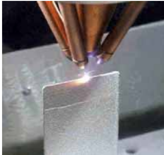
Figure 4: LENS Laser Head Heats Substrate While Powder Is Delivered Through Four Pressurized Nozzles
