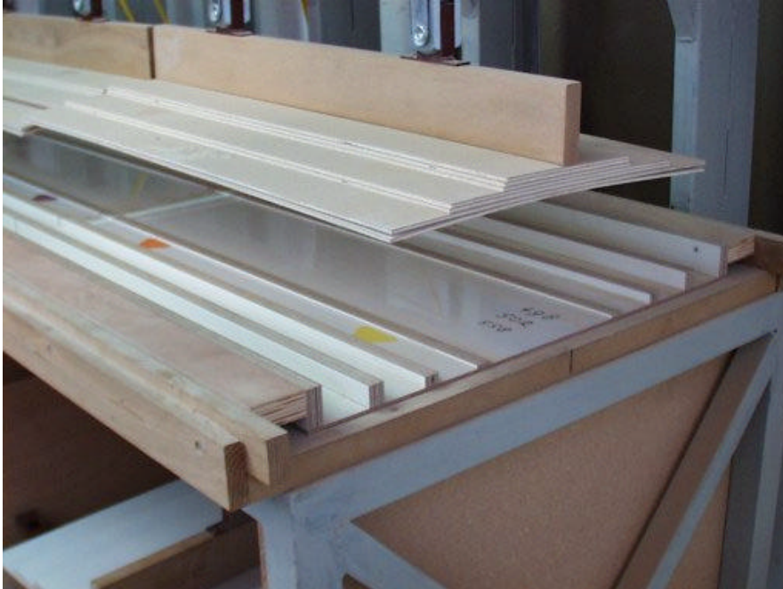
Pic-4 The new press -upper section of the press - leaf spring
