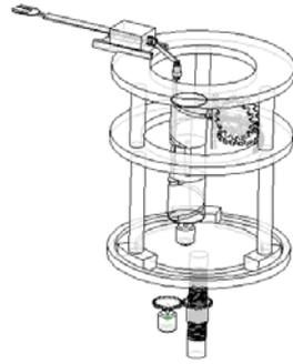
(a) The dual-cam mechanism
