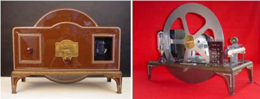
Fig.3. Television with the Nipkov disk.
