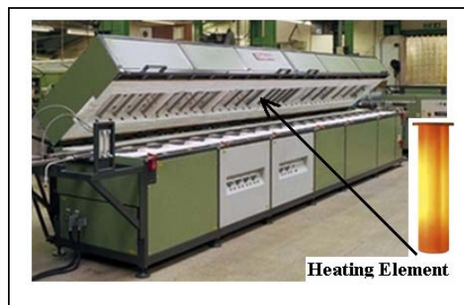
Figure 2: Stainless steel heat treating furnace.
